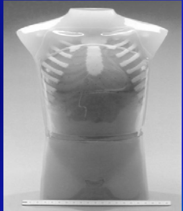
\*Intercalibration of in vivo counting systems using an Asian phantom, IAEA, 2003
